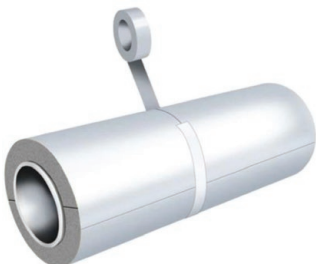
Figure 6 shows Saranex as the factory-applied vapor retarder. 1” or greater Saranex 520 tape should be used to wrap outside of the Saranex vapor retarder at 18” centers with 25% circumferential overlap (1 ¼ wraps).
