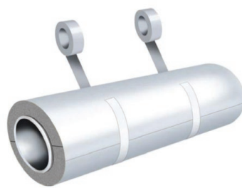
Figure 7 shows a vapor retarder other than Saranex as the factory-applied vapor retarder. 1” or greater Saranex 520 tape or ¾” or greater filament tape should be used to wrap outside of the vapor retarder at 12” centers with 25% circumferential overlap (1 ¼ wraps).
